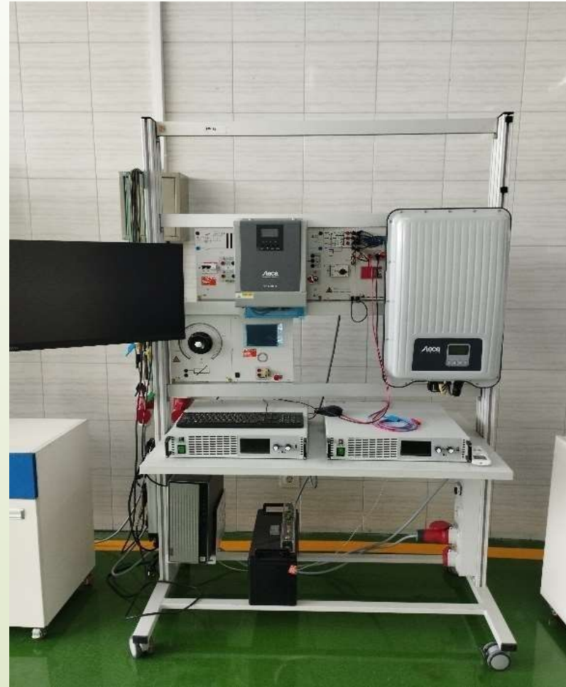
EIT 4.1 Photovoltaic Hybrid System with Battery
